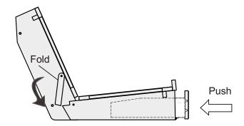
Yokohama in Sofa Position. Fold Leg Support to lock the Back Deck and Seat Deck as shown. Push the Drawer in.
