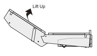
Until the Seat Deck fully down on the floor
