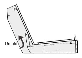
Unfold Leg Support to unlock the Back Deck and Seat Deck as shown.
